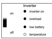
The inverter switched off due to excess ripple voltage on the battery terminals.
